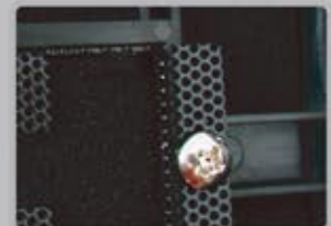
Metal mesh drive bay mounted solidly
